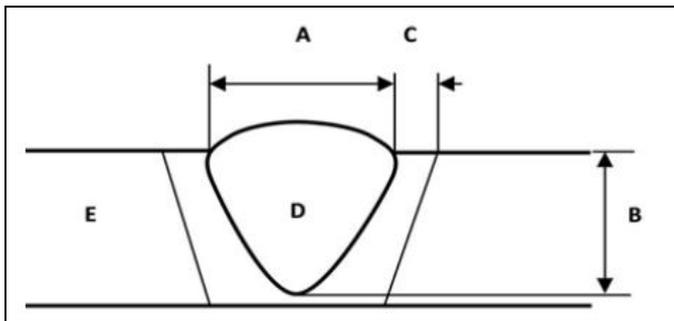
**Fig.1** Weld bead shape parameter. A: Bead width, B: Depth of penetration, C: HAZ width, D: Weld metal, E: Base metal.
