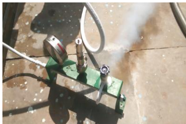
Fig 5.4: Pressure Gauge – Globe valve setup
