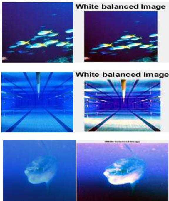
Fig-3: Input images with white balanced output images.
