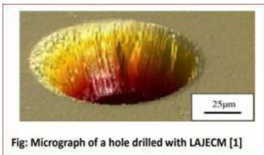
Fig: Micrograph of a hole drilled with LAJECM [1]
