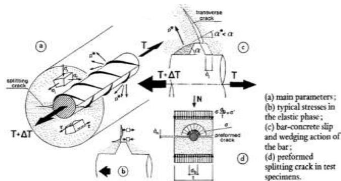
Fig -3: Bond and splitting in reinforced concrete
