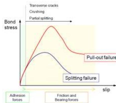
**Fig -7.2:** Bond stress vs. slip behaviour of deformed bars
