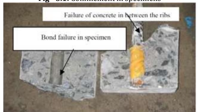
Fig -5.2: Splitting failure in specimens
