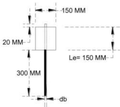
Fig -11.1: Details of pull out specimen
