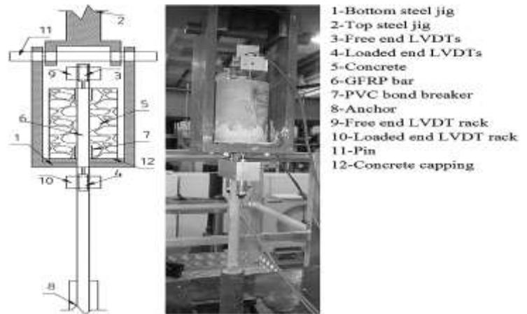
Fig -9: Set up of pull out test
