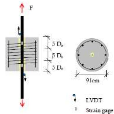
**Fig -7.1:** Details of test specimen
