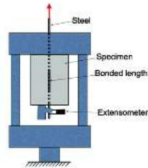
Fig -1.1: Pull out test set up
