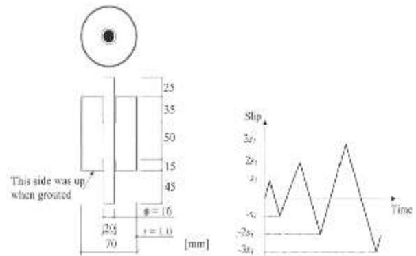
Fig -4: Geometry and c/s of test specimen
