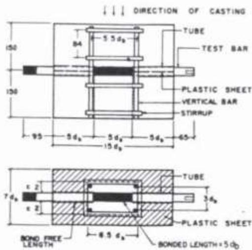
Fig -2: Test specimen
