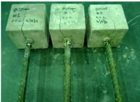
Fig -11.2: Pull out specimen after testing
