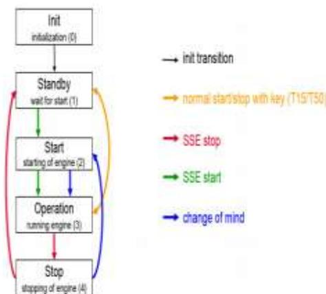
Fig-2: State diagram of ISG
