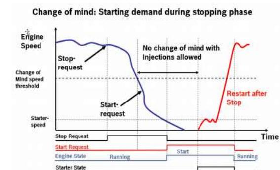
Fig-4: Change of mind when Engine Speed < Threshold
