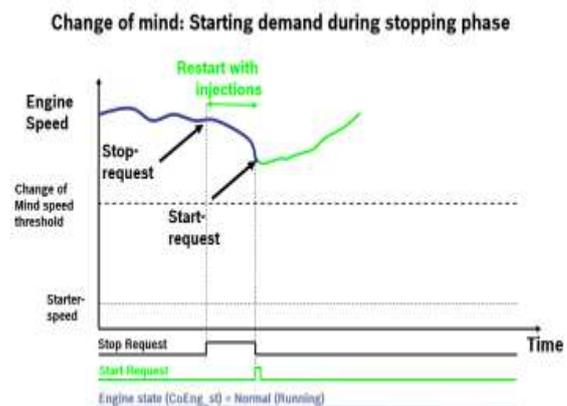
Fig-3: Change of mind when Engine Speed > Threshold
