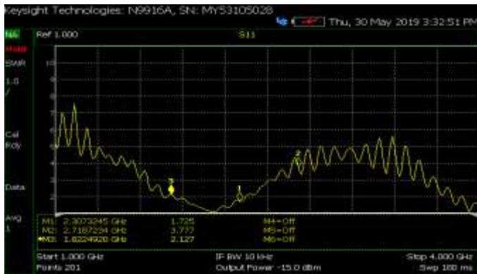
Fig -9: Measured VSWR versus frequency plot
