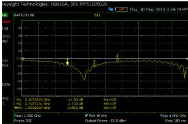
Fig -8: Measured reflection coefficient versus frequency plot
