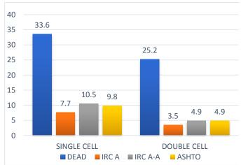
The above graph shows the displacement values for the all four load cases such as Dead load, IRC A, IRC A-A & Ashto codes.
