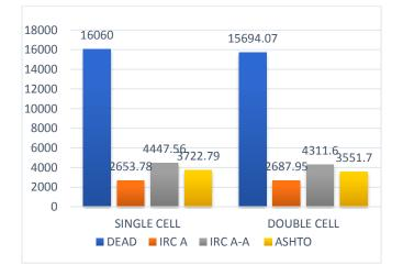
The above graph shows the Bending moments values for the all four load cases such as Dead load, IRC A, IRC A-A & Ashto codes.
