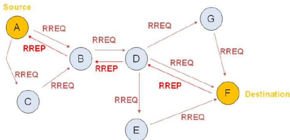
Fig- 2: Example of a AODV Routing Protocol
