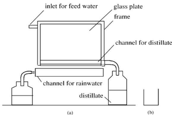
Figure1. (a)Elevation of the still; (b) cross section of the distillate channel.
