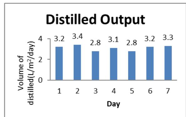
Figure3. Cumulative volume of distilled water (L/m<sup>2</sup>/day)
