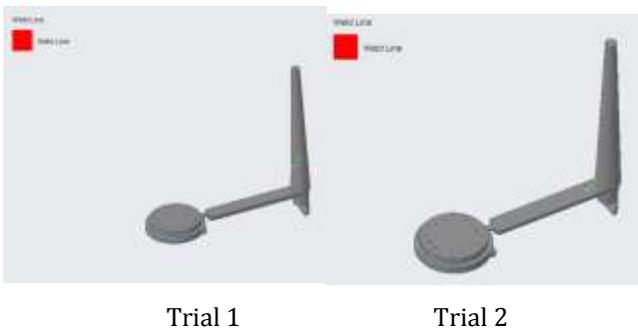
Figure 6. Weld line analysis for gas sensor
