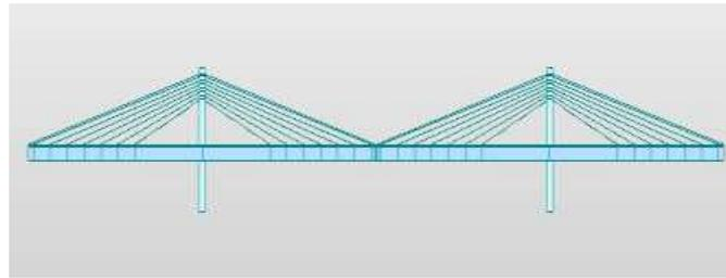
**Figure 1** Finite element representation of 144m long Extradosed Bridge
