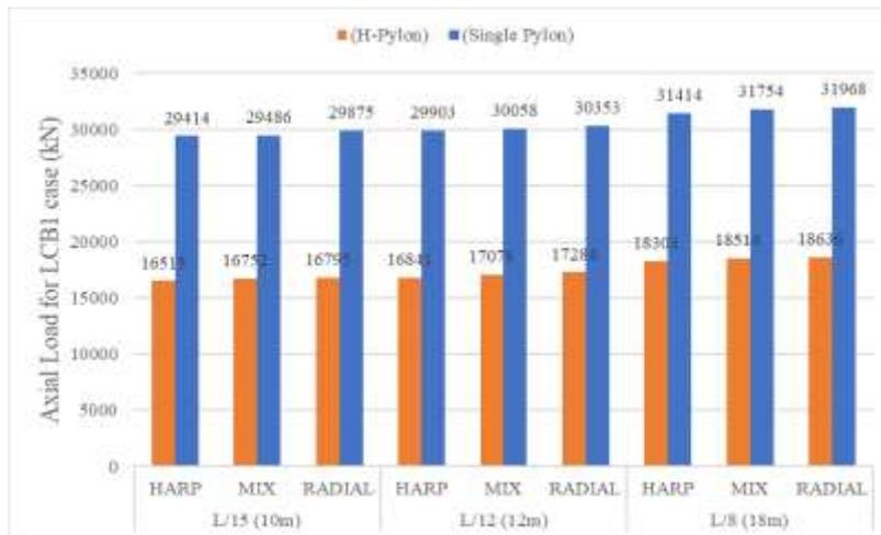
Figure 3 Comparison of Support Reaction for all the 18 cases
