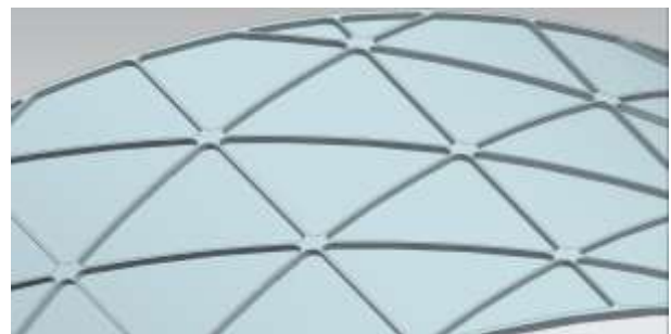
Fig -2: Iso-grid Stiffened patterns
