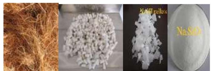
Fig 3: Materials ready to make a batch of fly ash based geo-polymer mortar
