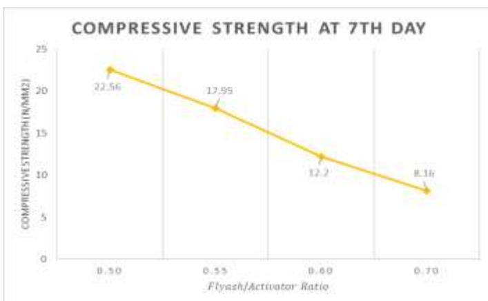
**Fig 7:** Compressive strength values of 7 days cured specimens of all ratios
