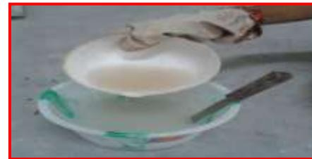
Fig 2: Mixing of  $\text{Na}_2\text{SiO}_3$  with NaOH
