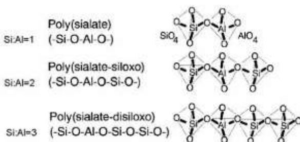
Fig 1: Three basic forms of geo-polymer
