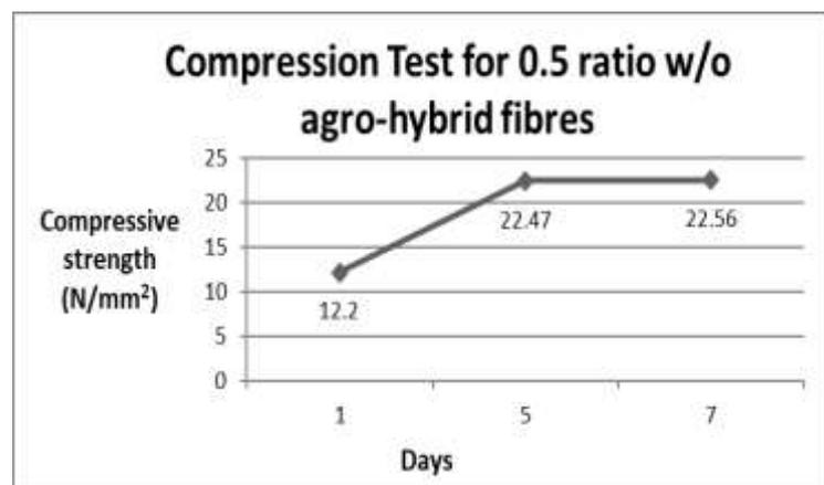
Fig 5: Compression test result for 0.5 ratio.
