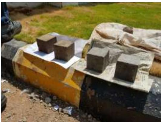
Fig4: Curing of Specimen
