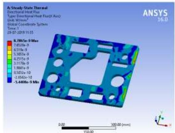
Fig:12. Directional Heat Flux (Steady State Thermal)
