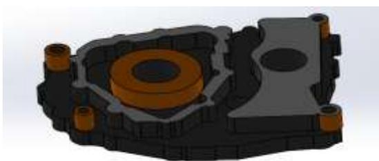
Fig 5. Crank Case right 3D model
