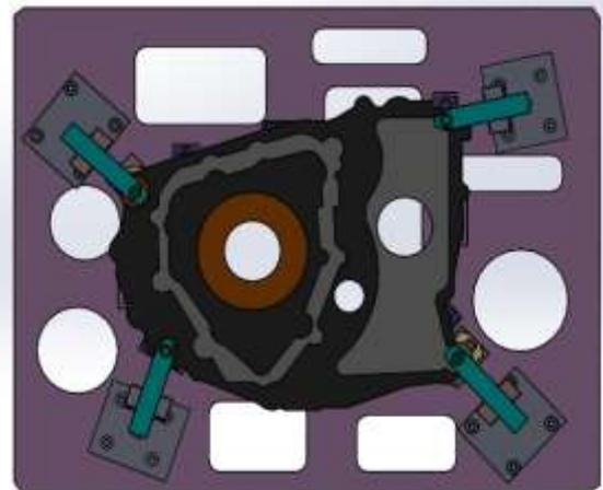
Fig 6. Shows 3D CAD model of Fixture Assembly of Crank Case right
