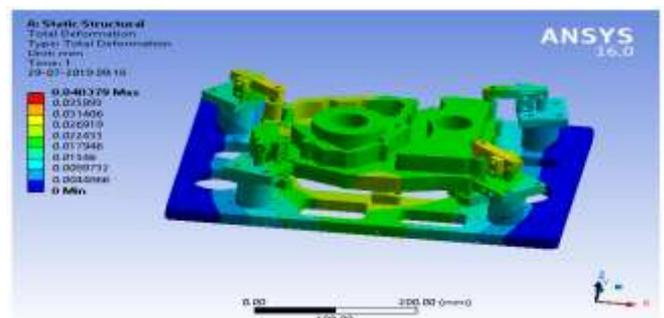
Fig: 11. Static Structural Total Deformation for 4bar
