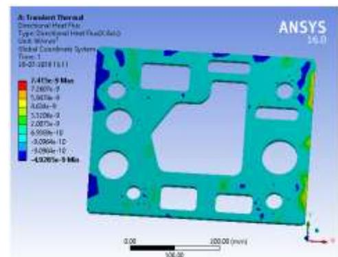
Fig: 14. Transient Thermal Directional Heat Flux.
