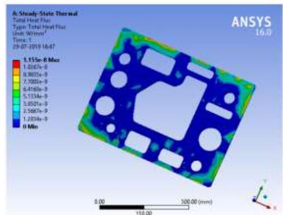
13. Total Heat Flux (Steady State Thermal)
