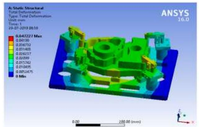
Fig: 9. Static Structural Total Deformation for 5bar
