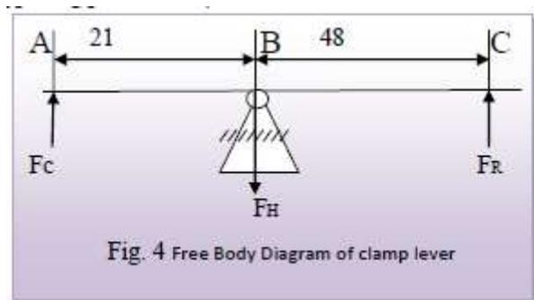
Fig. 4 Free Body Diagram of clamp lever
