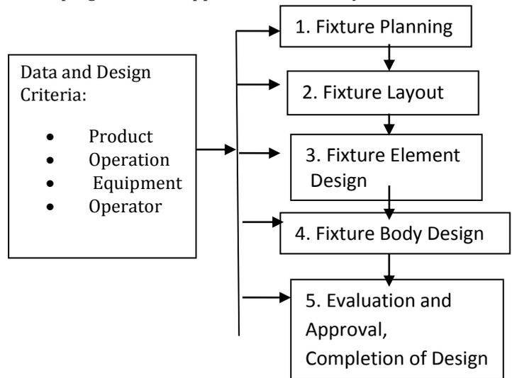
**Figure 1.4 various aspects of fixture design**
