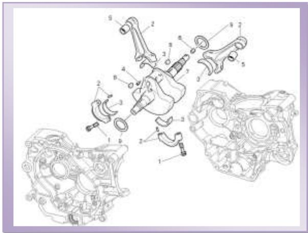
**Fig:2 Crank Case Assembly Drawing**
