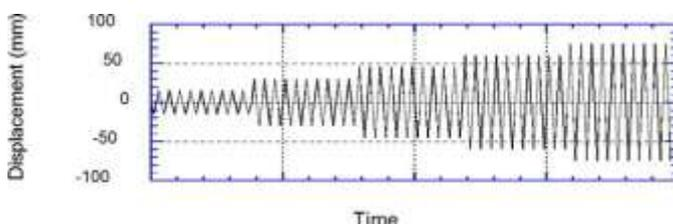
Fig-2: Displacement vs time graph of time history analysis
