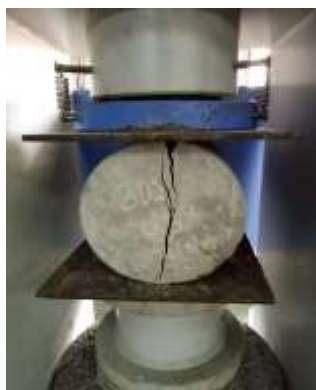
Fig -4 Cylinder testing using compression testing machine
