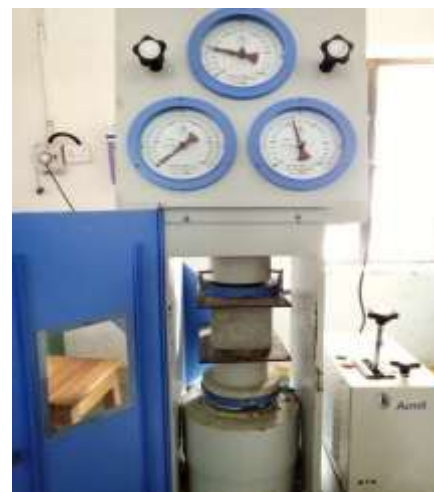
Fig -3 Cube testing using compression testing machine
