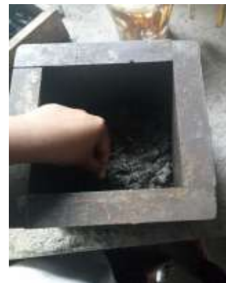
Fig -3 Placing steel fibres over concrete layer
