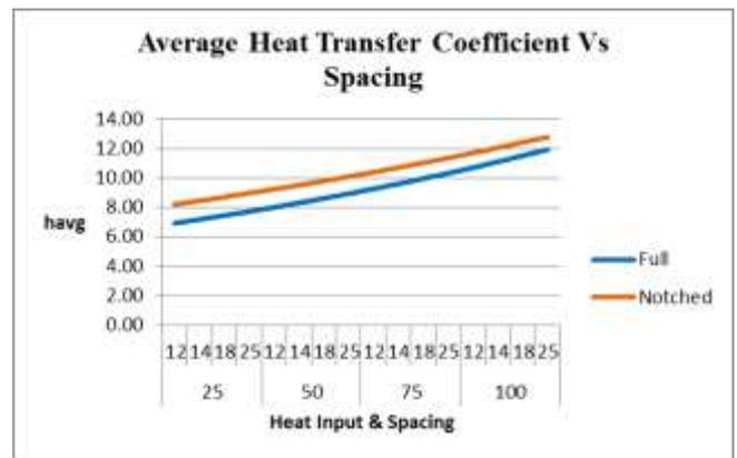
**Fig.6 Graph of Average heat transfer coefficients Vs spacing**
