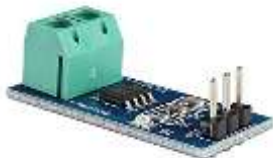
Fig -3: ACS712 20A current sensor
