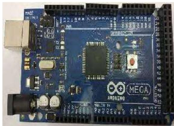
Figure 1 Arduino Mega 2560
