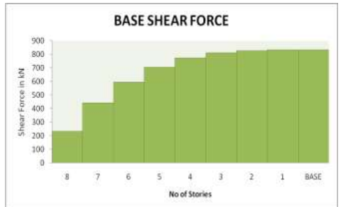
Fig. 7.3.a Base Shear for RCC Frame
