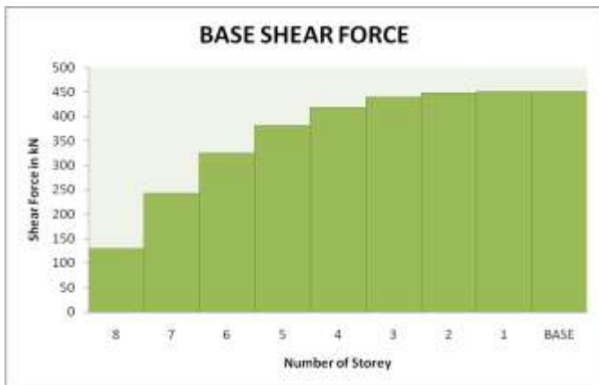
Fig. 7.3.c Base Shear for Composite Frame
