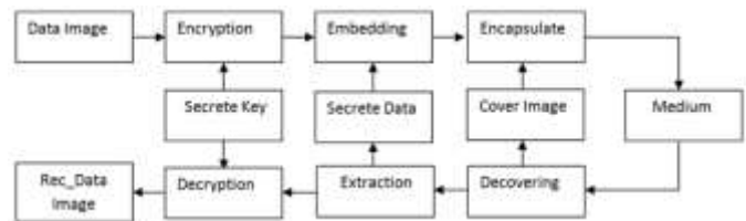
Fig(1): Schematic block diagram of the proposed VRAE reversible data hiding technique.
