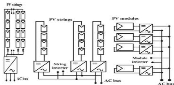
Fig -1: Configuration of PV Inverter
