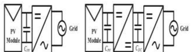
**Fig -4:** Capacitor Link Connection
