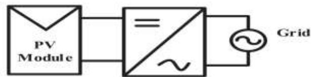
**Fig -2:** Single stage Inverter
