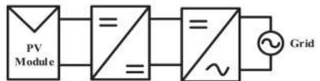
**Fig -3:** Multi stage Inverter
