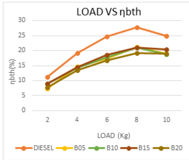
Fig 2: comparison of brake thermal efficiency for different blends
