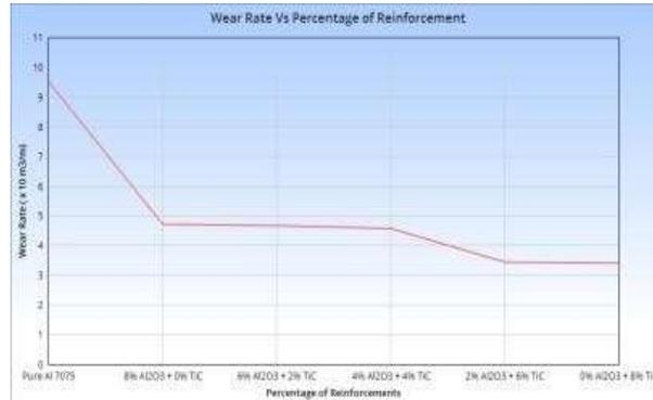
Figure 6: Wear rate Vs Percentage Reinforcements
