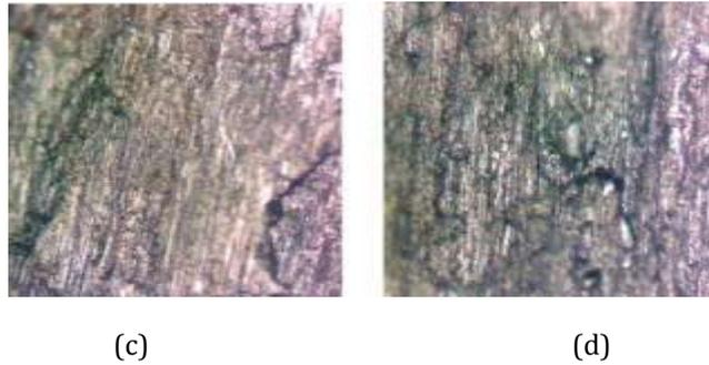
Figure 4: Microstructural images of worn surface – Al- 7075 with 8% TiC and 0 % Al<sub>2</sub>O<sub>3</sub> composition (100X)
