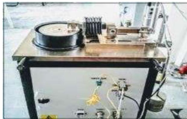
Figure 2: Pin-on-Disc Machine
