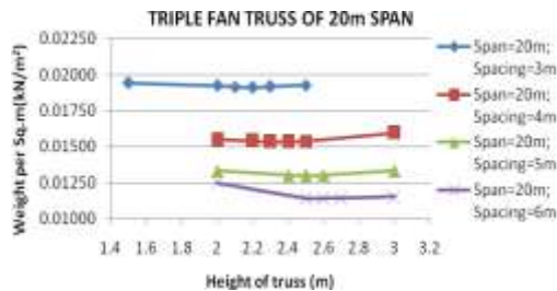
Chart 9: Plot of weight per m 2 v/s rise of 20m triple fan
