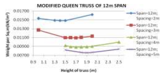
Chart 12: Plot of weight per m 2 v/s rise of 12m modified queen truss
