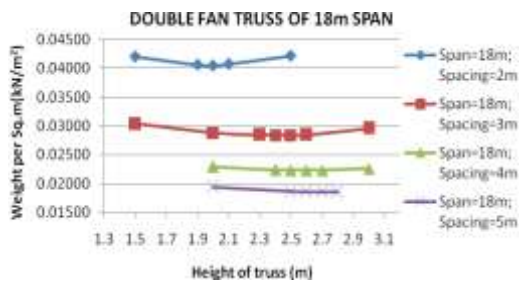
Chart 4: Plot of weight per m 2 v/s rise of 18m double fan
