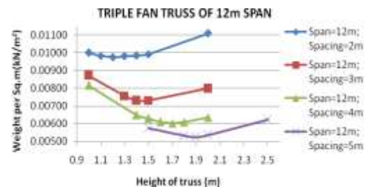
Chart 6: Plot of weight per m 2 v/s rise of 12m triple fan
