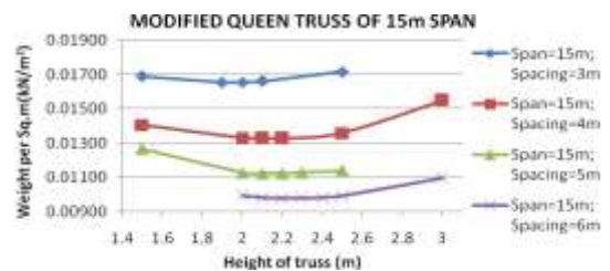
Chart 13: Plot of weight per m 2 v/s rise of 15m modified queen truss
