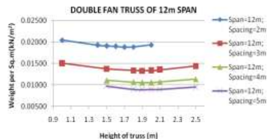
Chart 2: Plot of weight per m 2 v/s rise of 12m double fan
