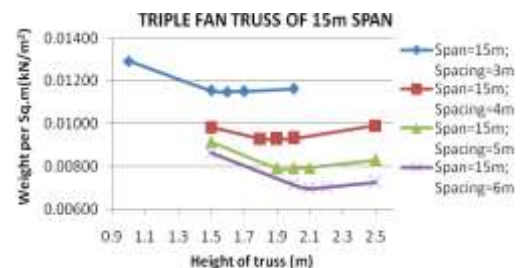
Chart 7: Plot of weight per m 2 v/s rise of 15m triple fan
