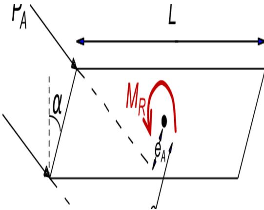
Fig: Rotational movement of abutment
