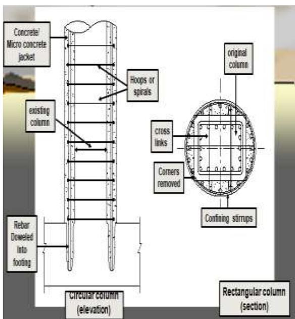
Fig.: CONFINEMENT OF COLUMNS BY CONCRETE JACKETING
