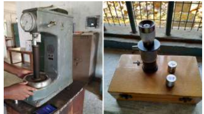
Fig: 8 Hardness Testing Machine and Microscope
