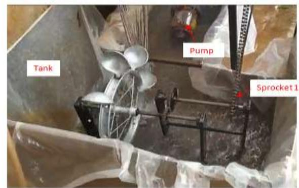
**Fig-2:** Turbine and gear drive in motion
