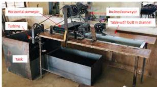
**Fig-5:** Isometric view of the machine
