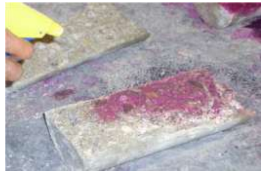
Fig-11: Carbonation Test
