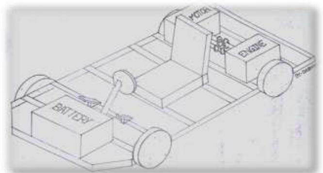
**Fig -6: Diagram of Components Arrangement**
