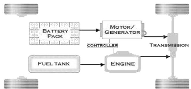
Fig -1: Parallel Hybrid Arrangement
