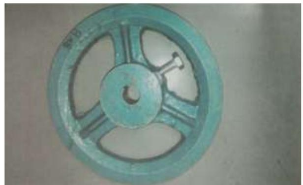
Fig- 6: Large Pulley
