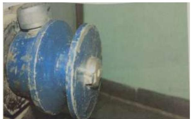
Fig- 7: Small Pulley
