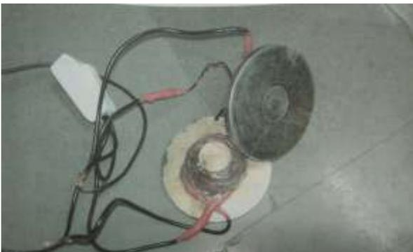
Fig- 3: Electromagnets
