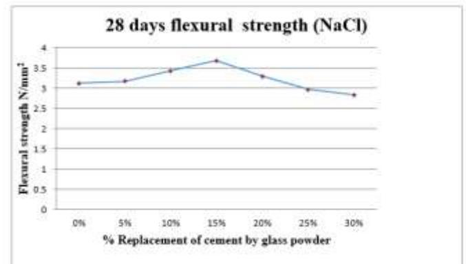
Chart-12: 28 days flexural strength of concrete when immersed in 5% NaCl solution
