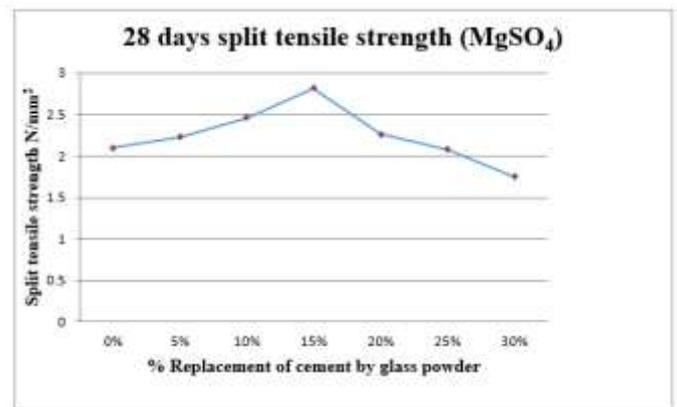
Chart-11: 28 days split tensile strength of concrete when immersed in 5% MgSO<sub>4</sub> solution
