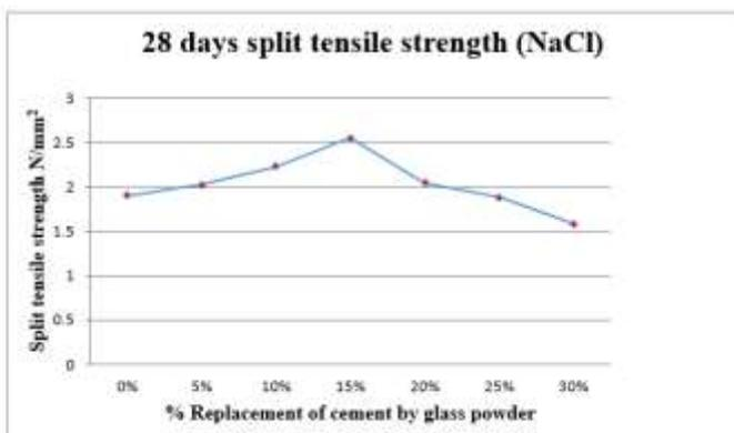
Chart-10: 28 days split tensile strength of concrete when immersed in 5% NaCl solution
