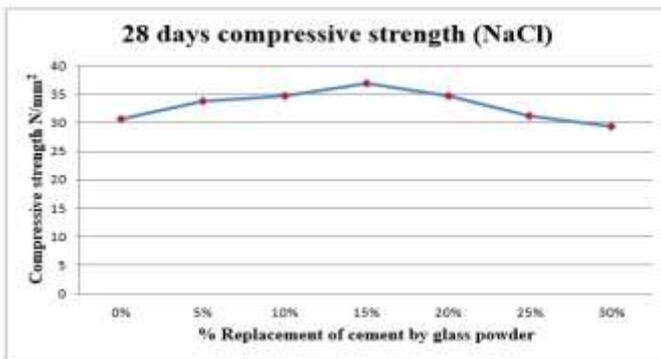
Chart-8: 28 days compressive strength of concrete when immersed in 5% NaCl solution
