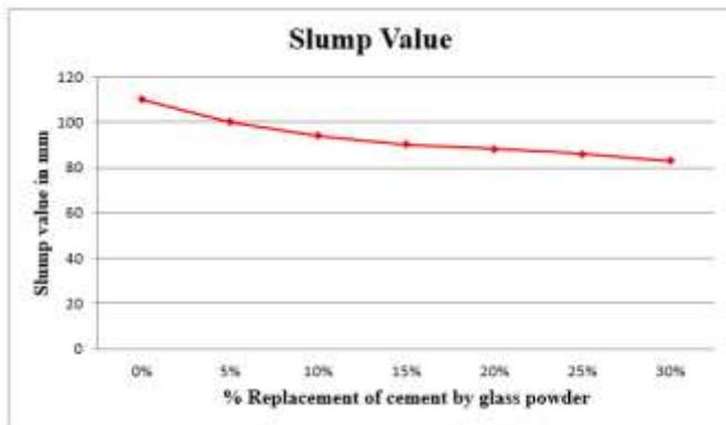
**Chart-1: Slump value for % replacement of cement by glass powder**
