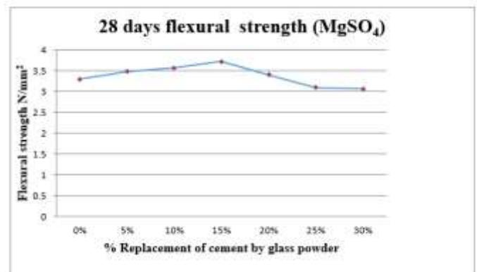
Chart-13: 28 days flexural strength of concrete when immersed in 5% MgSO<sub>4</sub> solution
