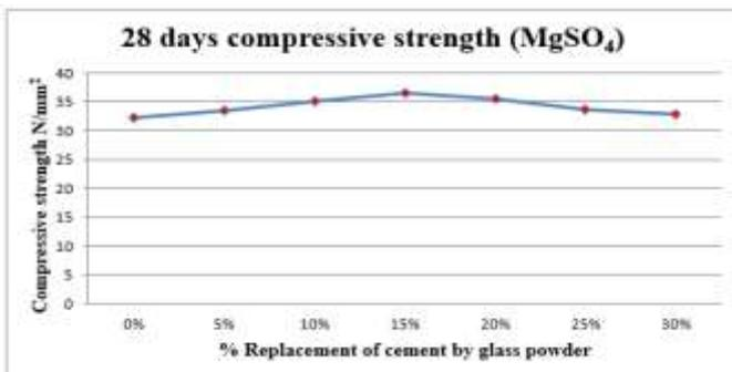
Chart-9: 28 days compressive strength of concrete when immersed in 5% MgSO<sub>4</sub> solution
