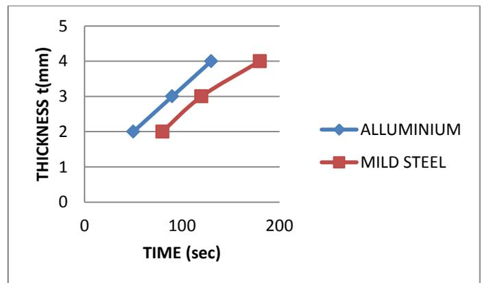
The thickness v/s time graph for length 1220mm of both Aluminium and Mild steel test specimen
