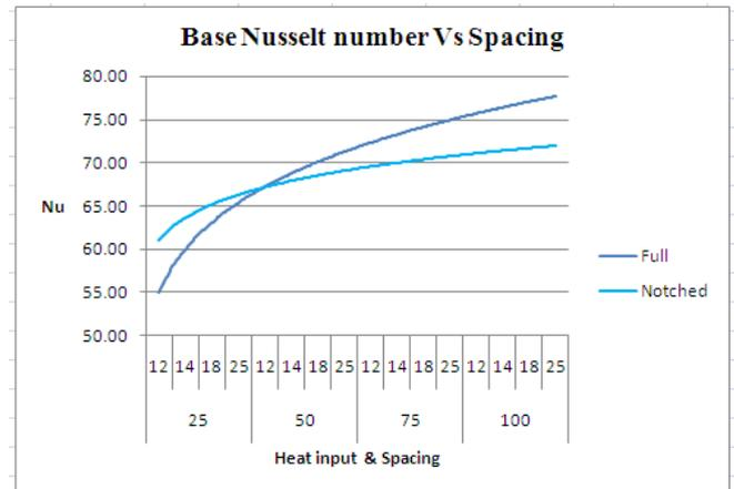
**Fig.5 Graph of Base Nusselt number Vs Spacing**
