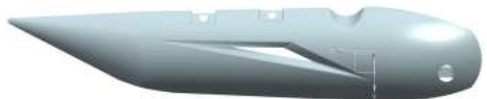
Fig-6- Modified design of muffler guard with Cutting Edge
