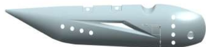
Fig-8- Final Proposed design of muffler guard with Vertical, Horizontal Holes and Cutting Big End
