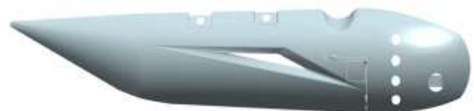
Fig-7- Modified design of muffler guard Vertical Hole with Cutting Edge
