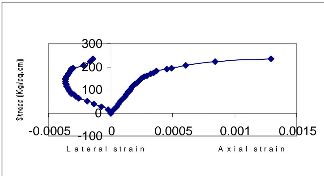
Figure 3 Stress-strain Behaviour of concrete cylinder C2 (5)
