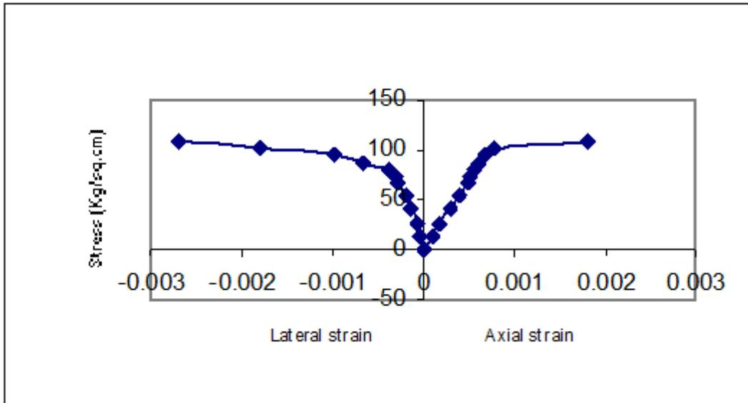
Figure 2 Stress-strain Behaviour of concrete cylinder C2 (4)
