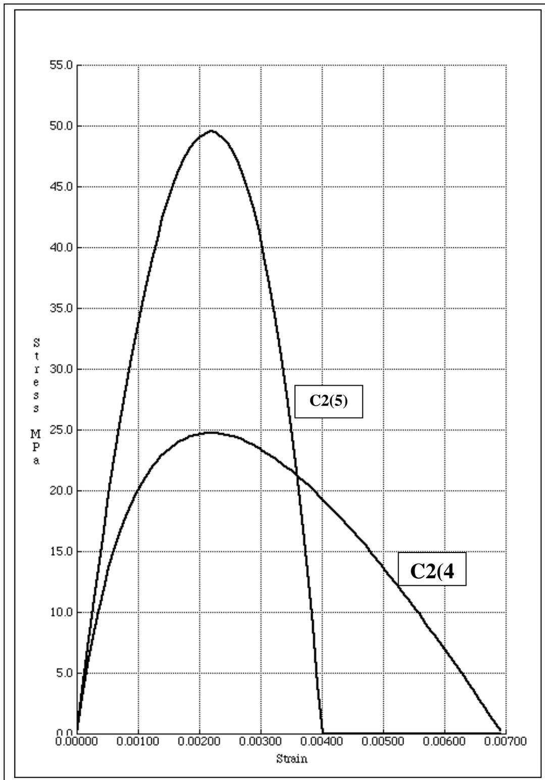
Figure 4 Behaviour of concrete cylinders C2 (4) and C2 (5) under controlled strain condition
