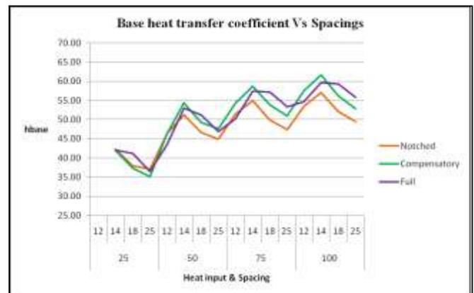
Fig.7 Graph of Base Heat Transfer Coefficient Vs Fin Spacing
