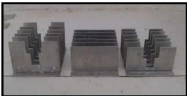
Fig.3 Assembly of Rectangular fin array
