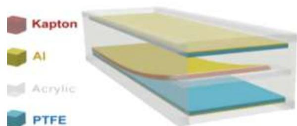
The breakdown of a TENG used to power LEDs [1]
