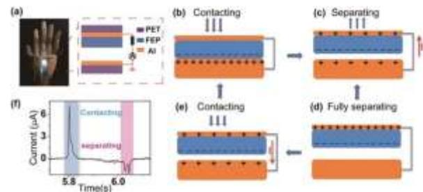
Fig(a) shows the physical model of the triboelectric nanogenerator and its placement on the artificial hand. Fig(b), (c), (d) and (e) show the cycle of charging and discharging. Fig(f) shows a graph, of the current readings obtained from the process [2].
