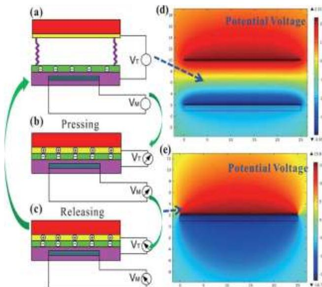
The working principle of the hybrid EMG and TENG: (a) the initial or separation mode; (b) the contact mode for pressing; (c) the contact mode for releasing; (d) the FEA simulation of the potential voltage with a 1 cm gap from the electret PTFE; and (e) the FEA simulation of the triboelectric potential voltage with a small gap.
