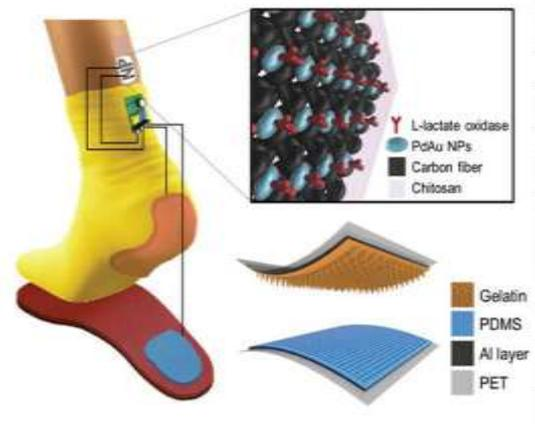
Schematic diagram showing a triboelectric nanogenerator-based lactate sensor. (© Wiley-VCH Verlag) [8]
