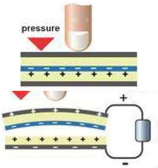
Simple production of current using static charges
