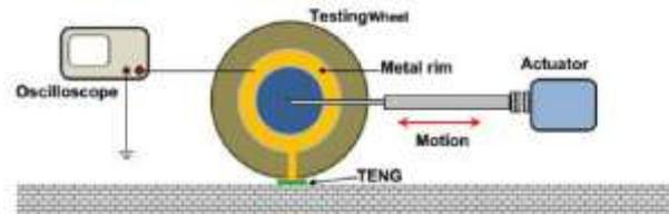
Schematic setup of characterising of the friction energy scavenging ability of the TENG from a rolling wheel [2]
