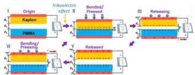
Vertical contact-separation mode of triboelectric nanogenerator
