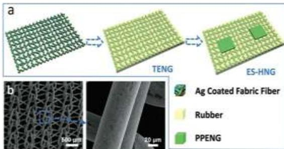
Fig(a) shows a normal textile being placed with TENGs creating a hybrid nanogenerator (HNG)
