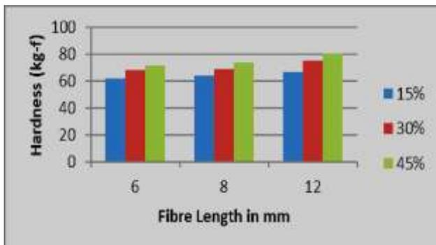
**Fig -3:** Effect of fiber parameters on Hardness of composites [35]
