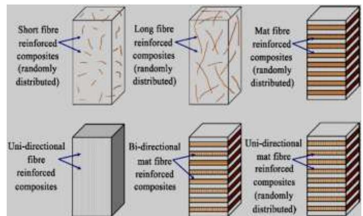
**Fig -1** Different type of fiber orientation used for laminate manufacturing [18]
