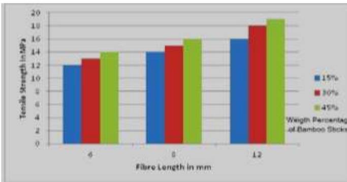
**Fig -2:** Effect of fiber parameters on tensile strength [35]
