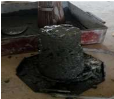
Fig-4: Slump cone test
