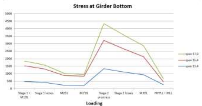
Chart 2: Stress at Girder Bottom comparison between span
