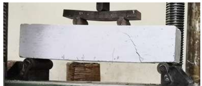
Fig. 3 cracking pattern of the steel-reinforced beam
