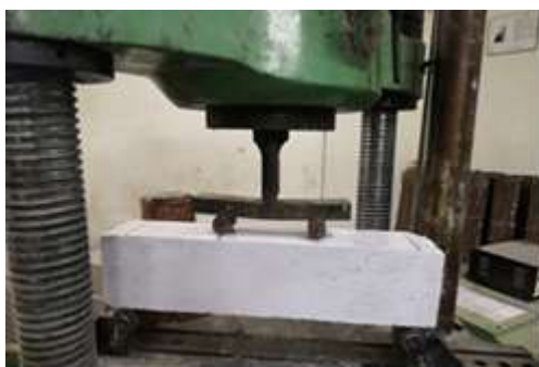
Fig. 2 setup for four-point bending test
