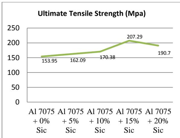
Fig: 8: Variation of Ultimate Tensile Strength
