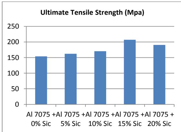
Fig: 7: Comparison of Ultimate Tensile strength
