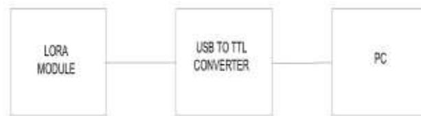
Fig-4. Block Diagram of sink node.
