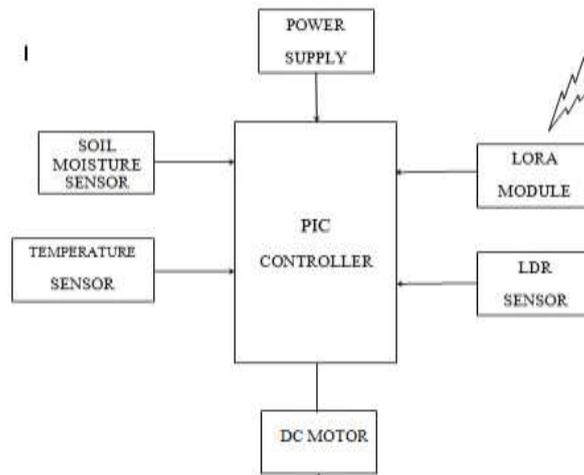
Fig-6. Block Diagram of Sensor Node.
