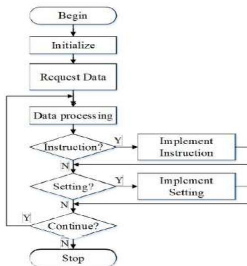
Fig-5 Flowchart of sink Node
