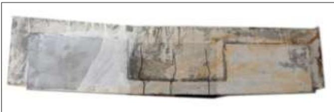
**Fig -16:** Crack pattern of GTRPM retrofitted beam (Partial U as end anchorage)
