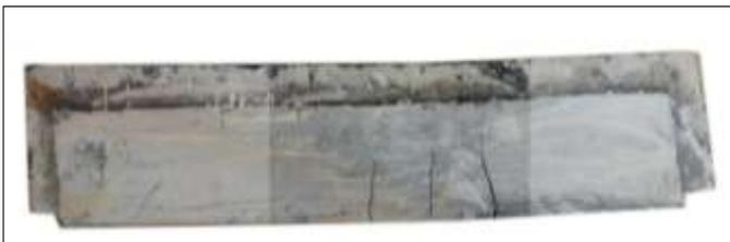
**Fig -17:** Crack pattern of GTRPM retrofitted beam (Partial U)
