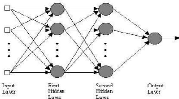
Fig -1:.Multiplayer perceptron (MLP with two hidden layer).
