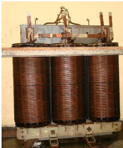
Fig. 1 Core assembly out of tank
