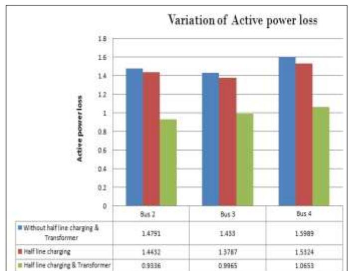
**Fig 5.** Graphical Representation of Variation of Active Power Loss with Half line charging & Transformer
