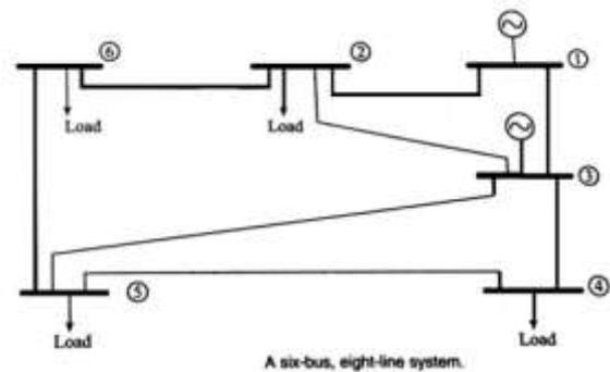
Fig 2. 6 bus 8-line transmission network.
