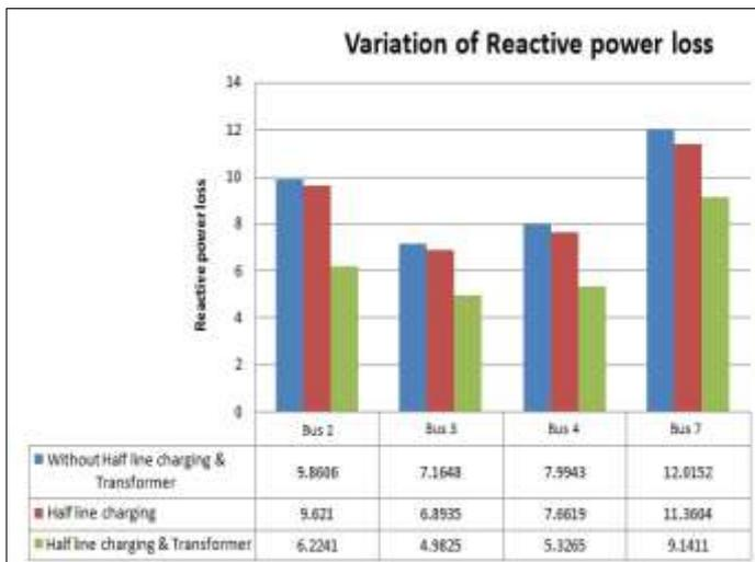
**Fig 6.** Graphical Representation of Variation of Reactive Power Loss with Half line charging & Transformer
