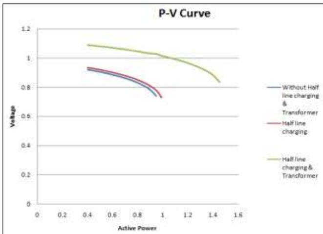
**Fig 8.** P-V curve considering different configuration.
