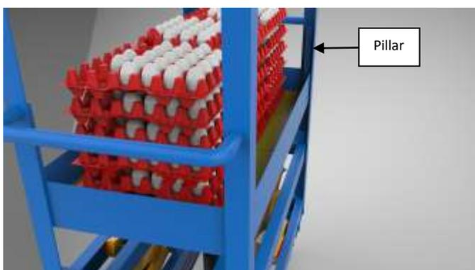
Fig. (10): Pillars for supporting Hopper 1
